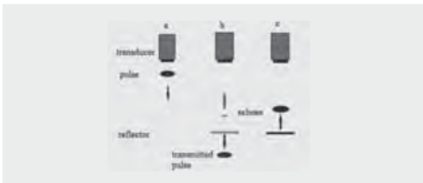
Fig. 1.2. Specular reflection. (a) Transducer emitting an ultrasound pulse. (b) Normally, most of the energy is transmitted at biological interfaces. (c) Gas causes total reflection
