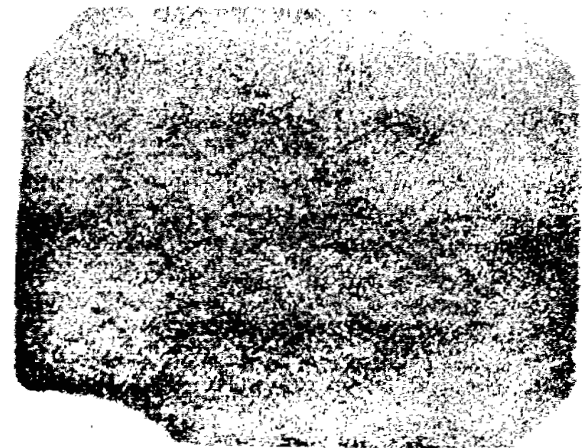
Figure 19.1. Burnt-out photomultiplier tube on field flood image.
