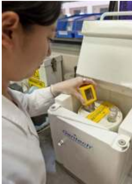
FIG. 9.9. Lead garage surrounding a ^{99}\text{Mo}/^{99\text{m}}\text{Tc} generator.
