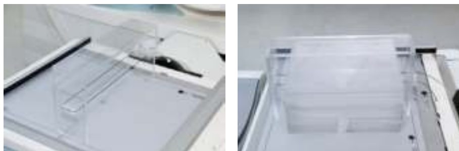
FIG. 15.4. A custom built, dual-line source phantom. On the left is the phantom positioned on the detector, and on the right the same line sources are immersed in a scattering medium consisting of sheets of Perspex.
