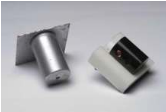
FIG. 15.1. Point source holders in a slanted position so that they can point to the detectors from the floor.
