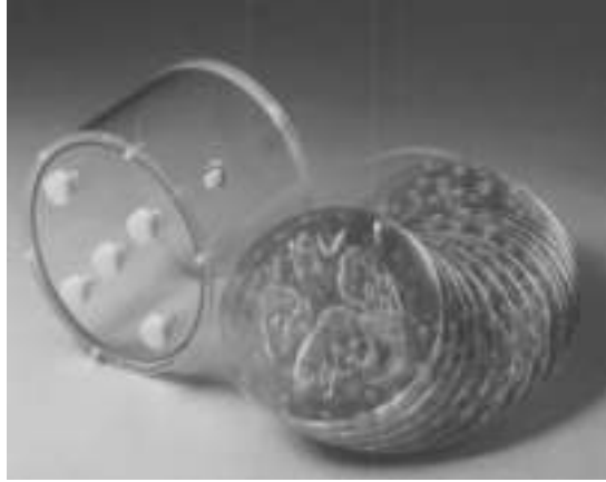
FIG. 15.14. Three dimensional Hoffman phantom with a water fillable cylinder and layers of inserts (phantom by Data Spectrum Corporation, USA).
