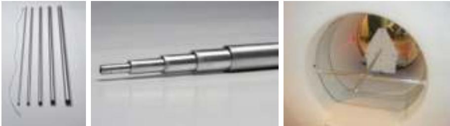
FIG. 15.20. Pictures of the National Electrical Manufacturers Association sensitivity phantom: positioning of the phantom within the gantry (right). A spring tensioned shower curtain rod and the point source holder are used to suspend the phantom within the field of view. The aluminium sleeves (left and centre) should coincide with the centre of the axial field of view.
