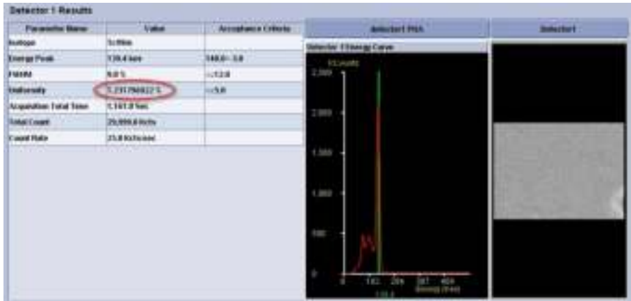
FIG. I.16. Routine intrinsic uniformity image with quantification. The image was obtained with a ^{99m}\text{Tc} point source, symmetrical energy window over 140 keV, 30 Mcounts. The image shows a hot semicircular area in the lower right field of view. The quantification indicates that the uniformity is acceptable. However, not indicated in the results, the uniformity calculation refers only to the central field of view. The artefact was due to a malfunctioning photomultiplier tube. Note: This camera required a service but could continue to be used with caution because of the lateral location of the defect. This example illustrates that it is essential to review together both image and quantification, and to understand the parameters provided in the results.
