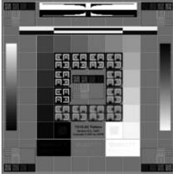
FIG. 14.19. Test pattern TG18-QC suitable for daily quality control of display monitor performance using visual inspection [14.13].
