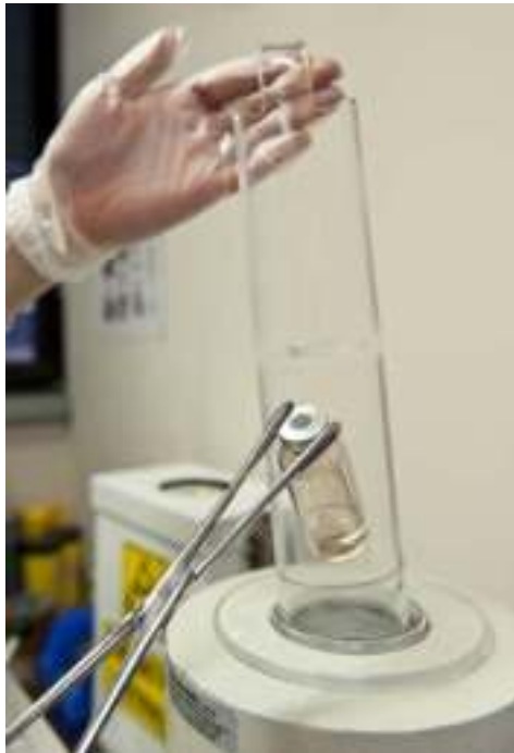
FIG. 9.11. Using long forceps to handle a vial containing radioactivity.
