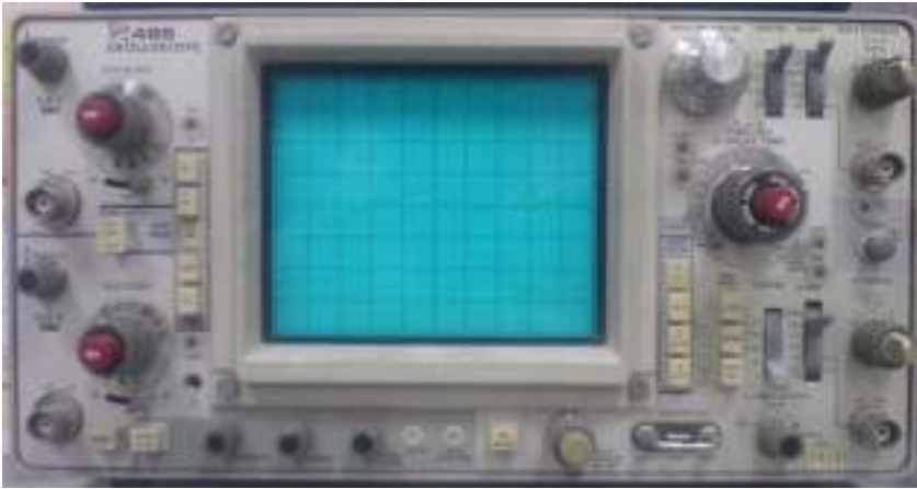
FIG. 7.16. The front panel of the Tektronix 465 oscilloscope.
