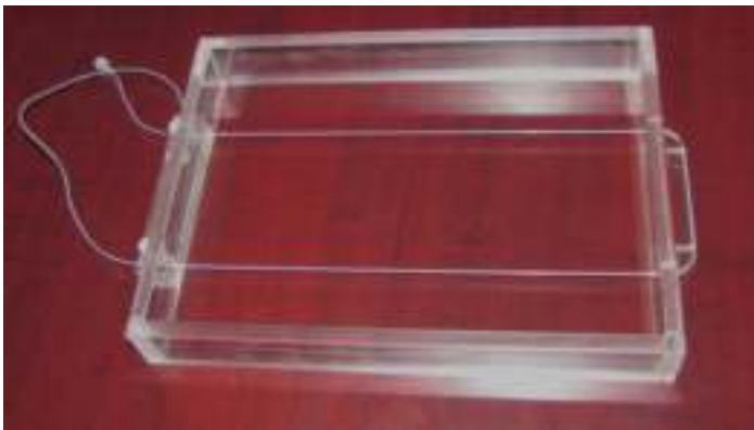
FIG. 15.6. Dual-line phantom for whole body resolution tests.
