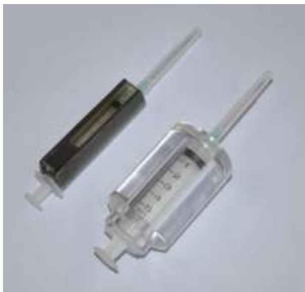
FIG. 9.12. A tungsten syringe shield for \gamma emitting radionuclides and a Perspex syringe shield for pure \beta emitters.
