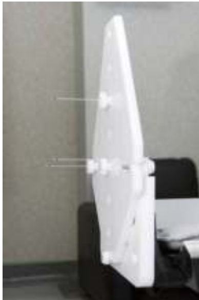
FIG. 15.22. Three capillary point sources mounted on a point source holder used in PET to measure spatial resolution.
