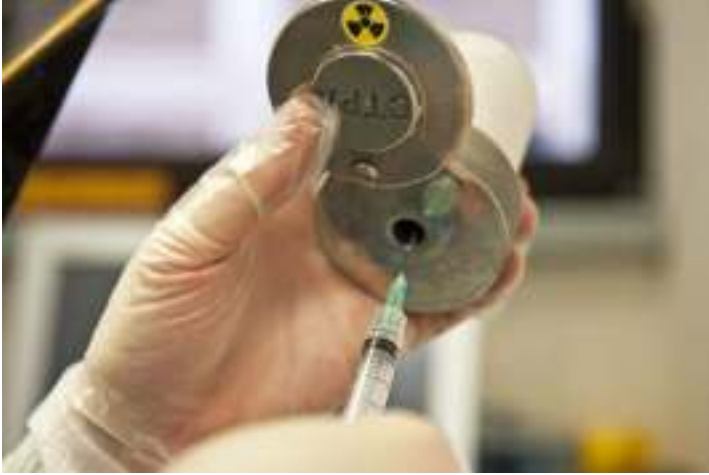
FIG. 9.10. Shielded vial used to hold reconstituted radiopharmaceuticals.
