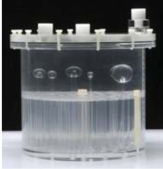
FIG. 15.12. Jaszczak phantom used for verifying image quality (phantom by Data Spectrum Corporation, USA).
