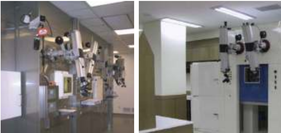
FIG. 4.17. Examples of modern hot-box designs (courtesy of Von Gahlen Nederland B.V.).
