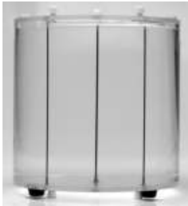
FIG. 15.10. A commercial triple-line source phantom with three line sources inside. The tank is filled with water to simulate a scattering medium.
