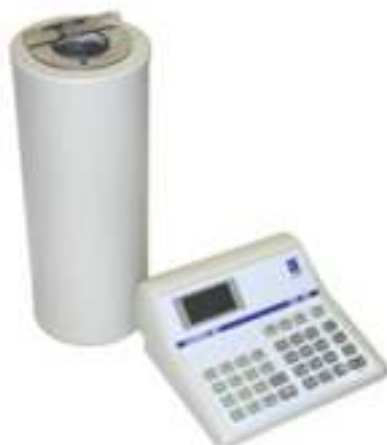
FIG. 9.1. A typical dose calibrator (e.g. CRC 25R).
