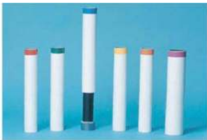
FIG. 10.8. Set of lead-lined plastic sleeves (Calichek™ Dose Calibrator Linearity Test Kit, Calichek, Cleveland, OH, USA) for evaluation of dose calibrator linearity by the shield method. The set is supplied with a 0.64 cm thick lead base, a colour coded unlined sleeve (to provide an activity measurement equivalent to the zero time point measurement of the decay method) and a six colour coded lead-lined sleeve providing attenuation factors nominally equivalent to decay over 6, 12, 20, 30, 40 and 50 h, respectively. (Courtesy of Calichek, Cleveland, OH, USA.)
