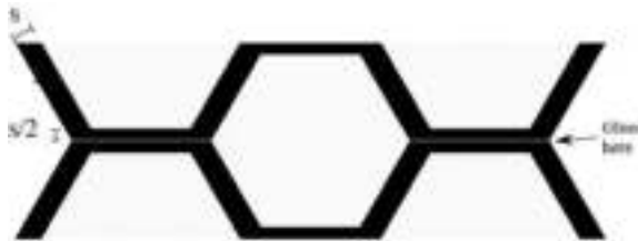
FIG. 11.5. Illustration of fabrication of foil collimator by gluing two stamped lead foils. It should be noted that the foils must be stamped so that the portions of the septa that are glued are half the thickness of the rest of the septa. Furthermore, careful alignment is essential to preserve the hole shapes.
