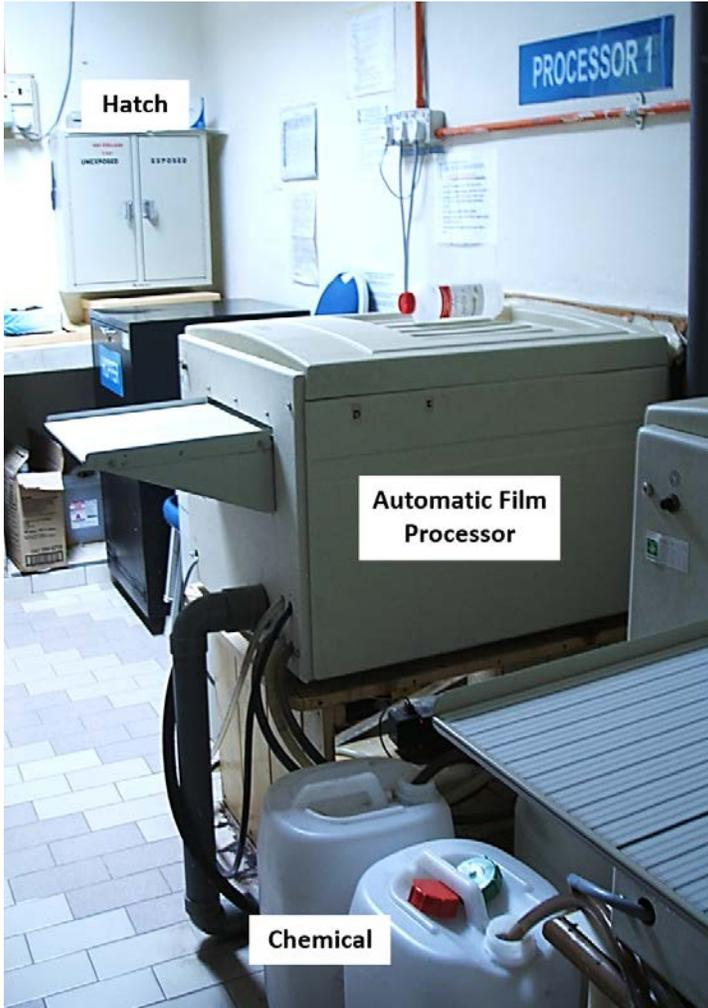
FIG. 23. Sample layout of a room for an automatic film processor. (Image courtesy of Chan Lai Kuan, Malaysia.)
